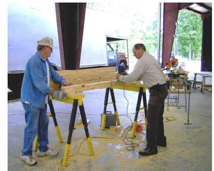
Ken held while Bud routed the bunk posts at another assembly line station.
